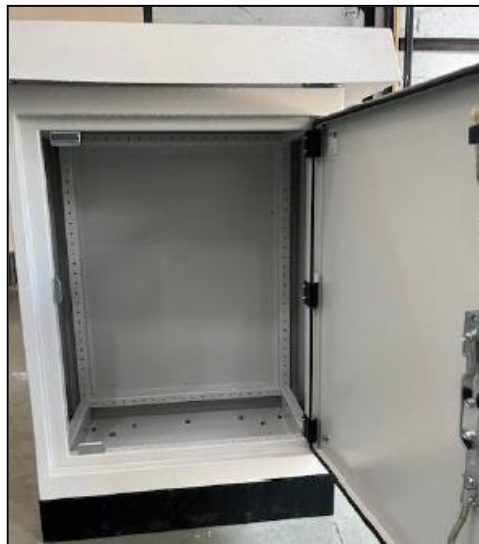
Fig 5 - After IP6X test (No ingress of dust observed)
