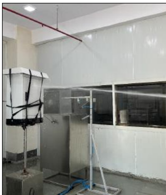
Fig 3 – IPX5 test setup
