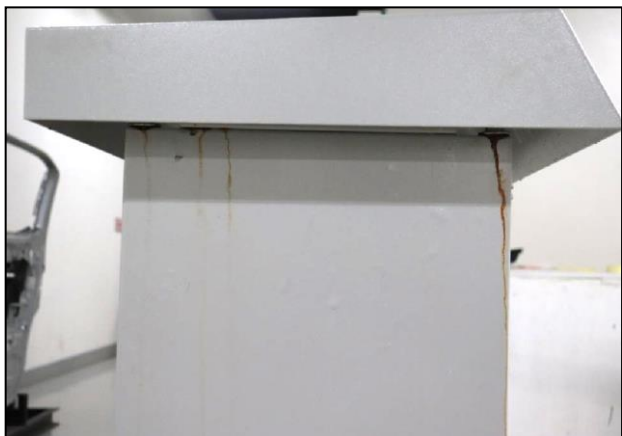
Fig 03 – DUT after the test (Red rust and coating ped off observed)
