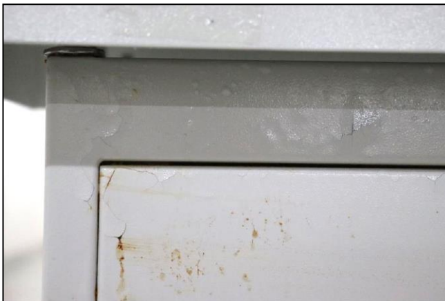
Fig 03 – DUT after the test (Red rust and coating ped off observed)
